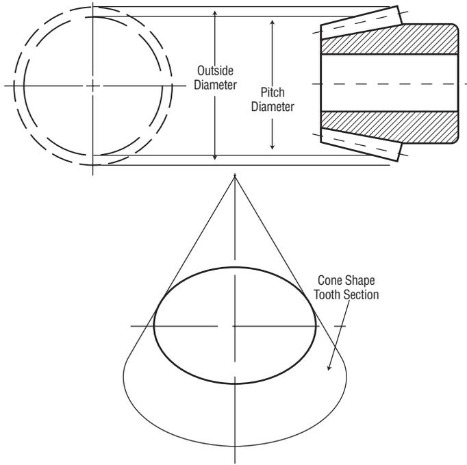
*Martin* stock bevel gear sets are designed to connect shafts that are on the same plane and at an angle of 90° to each other.
