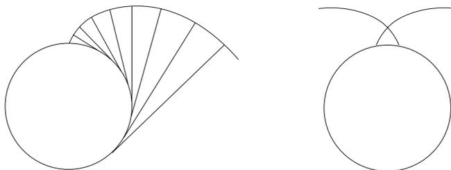
This tooth design reduces the sliding action of mating teeth thereby reducing friction and wear. It is formed by two involute curves drawn in opposite directions.
