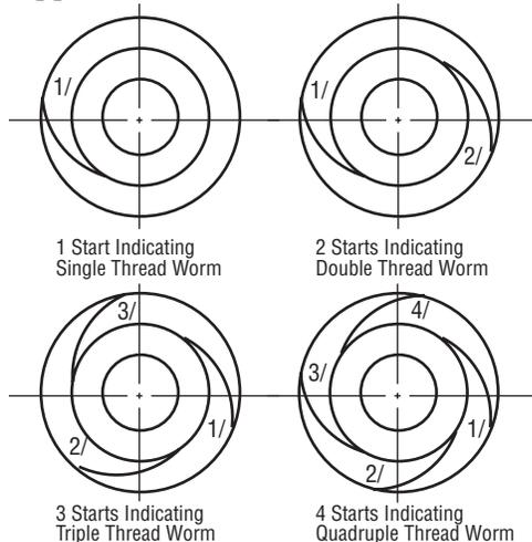
A stock worm may have one, two, three or four threads. The number of threads can be identified by counting the number of starts at the end.
