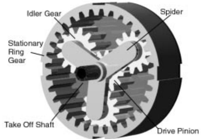
Planetary Gear Train with Driver, Driven & 3 Idlers
