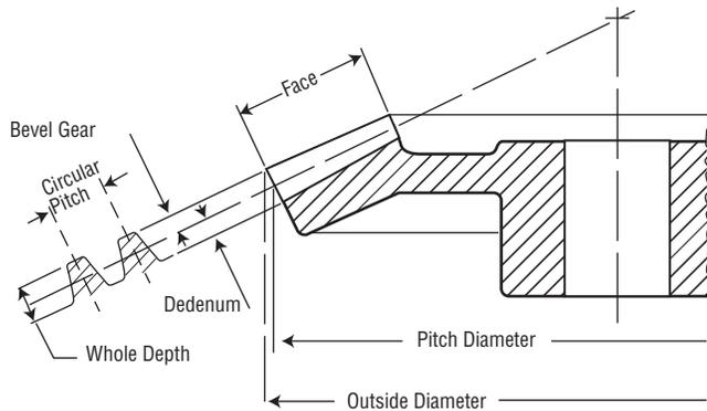
The Circular Pitch of a bevel gear may be found by measuring from a point on one tooth along the pitch line AT THE LARGE END OF THE TEETH to the same point on an adjacent tooth.
