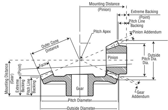
the pitch circle and the outside circle measured at the large end, or outside edge, of the tooth. It should be noted in this illustration that the pinion has a long addendum and the gear a short addendum while the whole depth of both are equal.
