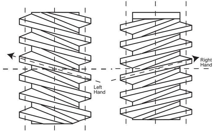
The number of threads on worms can be determined by looking at the end of the worm and counting the number of starts.
