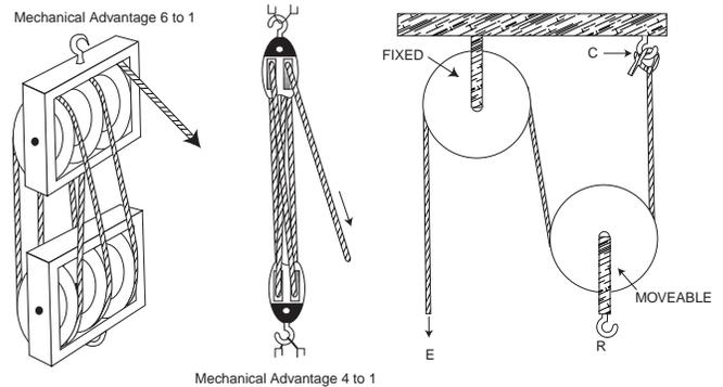
The second kind, by adding a moving pulley, cuts the effort in half to do the required work. The mechanical advantage is equal to the number of strands actually pulling the weight.
