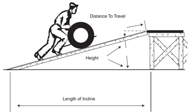
$$\text{FORCE} = \text{Load} \times \frac{\text{Length of Incline (LI)}}{\text{Height (H)}}$$
