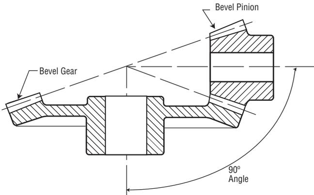
Since the bevel gear is always greater in pitch diameter and number of teeth than the bevel pinion, there is always a ratio greater than 1:1. It can, therefore, be said that a *Martin* bevel set is used to transmit power or motion at a 90° angle with a decrease
