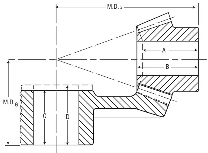
The illustration above shows the pinion having two lengths through bore (A & B), and gear having two (C & D), with pinion mounting distance (M.D.p) and gear mounting distance (M.D.G) remaining constant.
